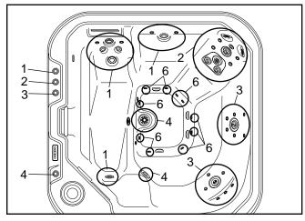
**Air Control 1** determines the amount of air flowing through the hydrotherapy jets labeled 1 in the drawing above. If the control is turned counterclockwise, the amount of air will increase; if the control is turned clockwise, the amount of air will decrease. Air controls 2, 3, and 4 function in the same manner.
